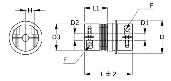
D = 109 Nom. torque NM (Tkn) = 200NM overload torque range 2 D1 = 45 Position engagement = C = Synchronous
